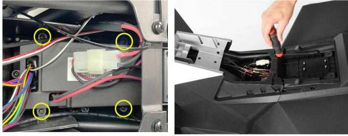
Step 6: Disconnect all nine connectors attached to the motor controller, by squeezing the tabs and pulling both ends.
