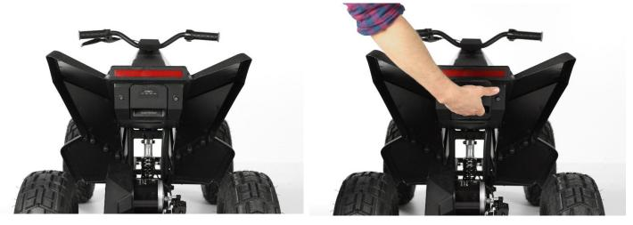
**Step 2:** Using a Phillips screwdriver, remove two screws within the battery housing.
