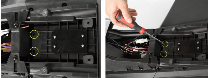
**Step 5:** Using a Phillips screwdriver, remove four screws fastening the motor controller to the body.
