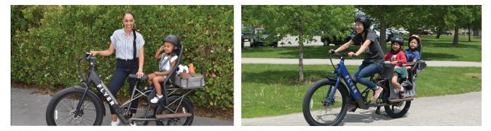
The Flyer L885 also sports fat tires just like the M880, but the rear 26-inch wheel gets swapped for a smaller 20-inch wheel to make room for more cargo and a lower center of gravity. We've seen this before with the RadWagon, though that bike lowered both wheel diameters to 22 inches to create a more nimble cargo e-bike with a lower center of gravity.
