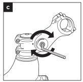
$\triangle$  WARNING! Overtightening the stem bolt can damage the handlebar stem assembly which can lead to risk of injury. To avoid overtightening, use a torque wrench and tighten to 16 Nm.
