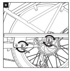
Step 10: Check fastener torque values
